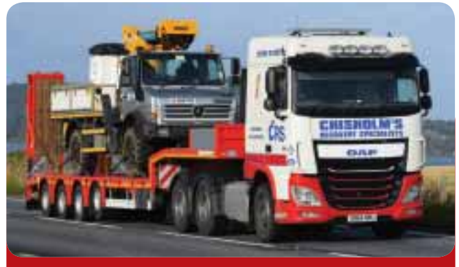
Chisholm's Recovery Specialist of Ballachulish and Inverness have taken a new Kassbohrer four axle extendable low loader with two rear self tracking axles and front lifting axle. Photo: Darren Green.
